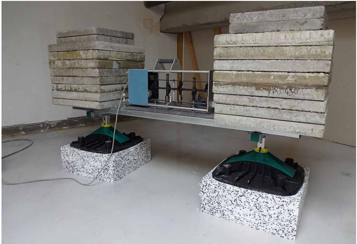
Photo 6: Measurement 5, BIS Yeti® Support System, type 480, 300 kg load per foot, with EPS-insulation
