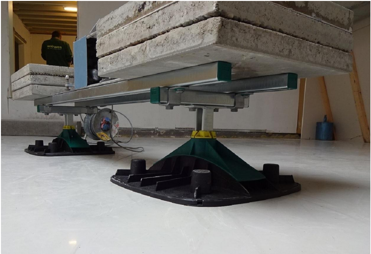
Photo 4: Measurement 2, BIS Yeti® Support System, type 480, 100 kg load per foot
