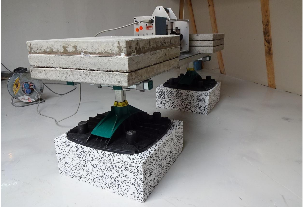
Photo 5: Measurement 3, BIS Yeti® Support System, type 480, 100 kg load per foot, with EPS-insulation
