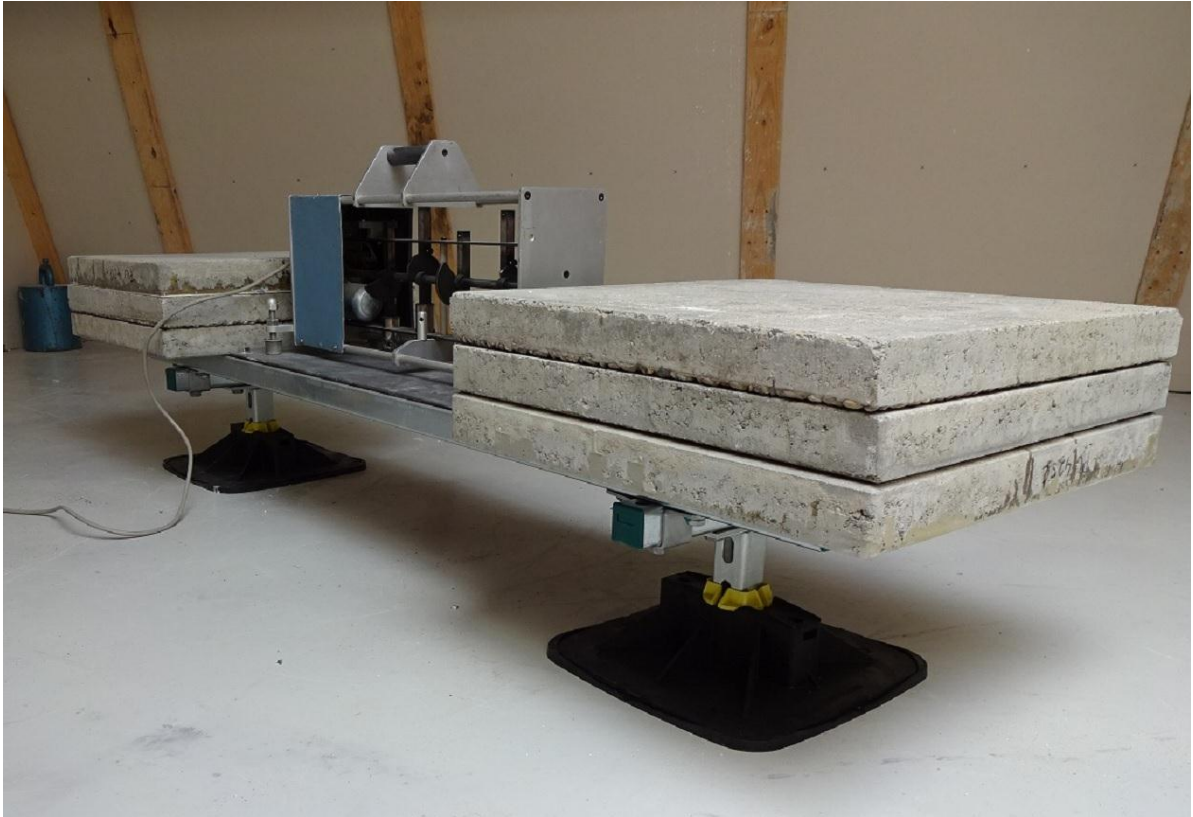
Photo 7: Measurement 6, BIS Yeti® Support System, type 335, 100 kg load per foot
