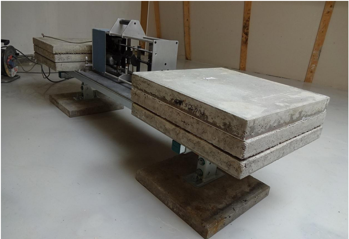
Photo 2: Reference construction, measurement 1, concrete slabs with rail base, 100 kg load per foot
