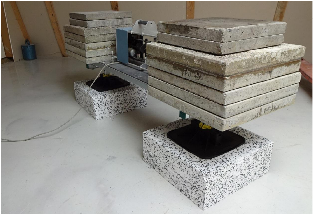
Photo 8: Measurement 8, BIS Yeti® Support System, type 335, 200 kg load per foot, with EPS-insulation
