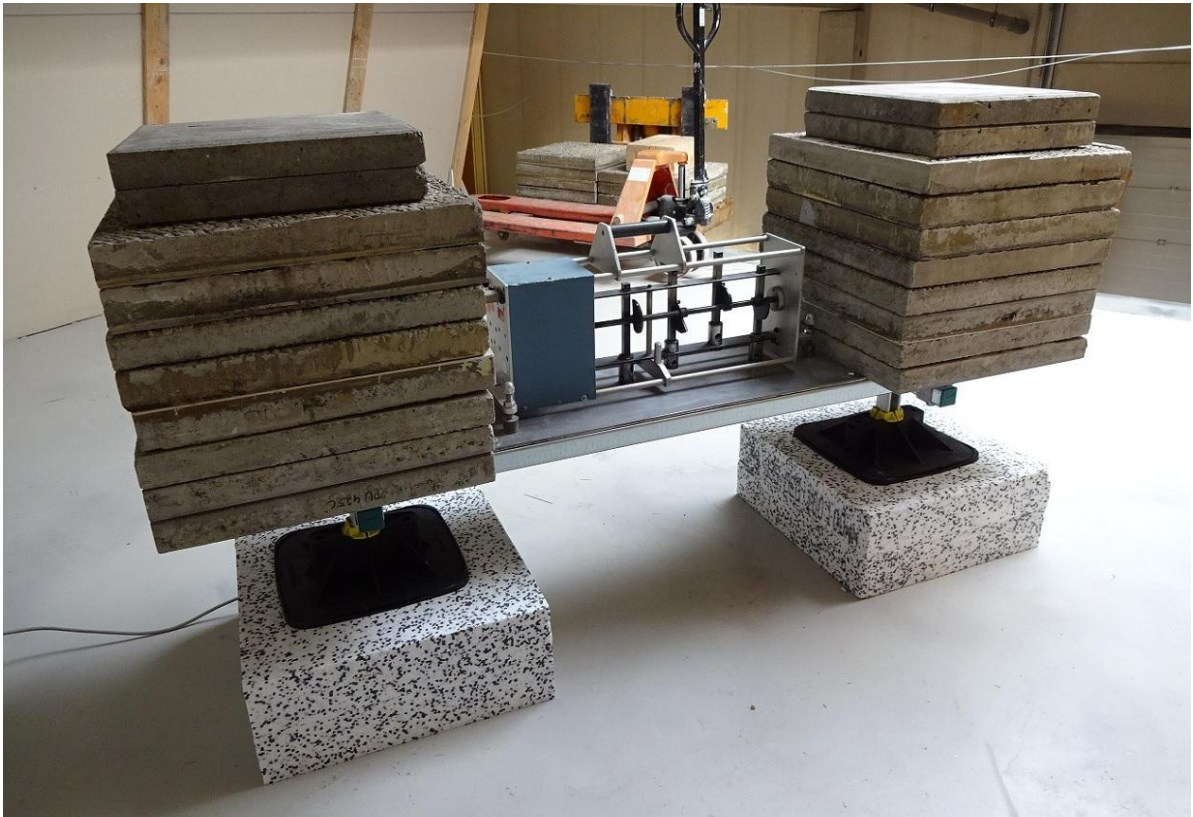
Photo 10: Measurement 9, BIS Yeti® Support System, type 335, 300 kg load per foot, with EPS-insulation
