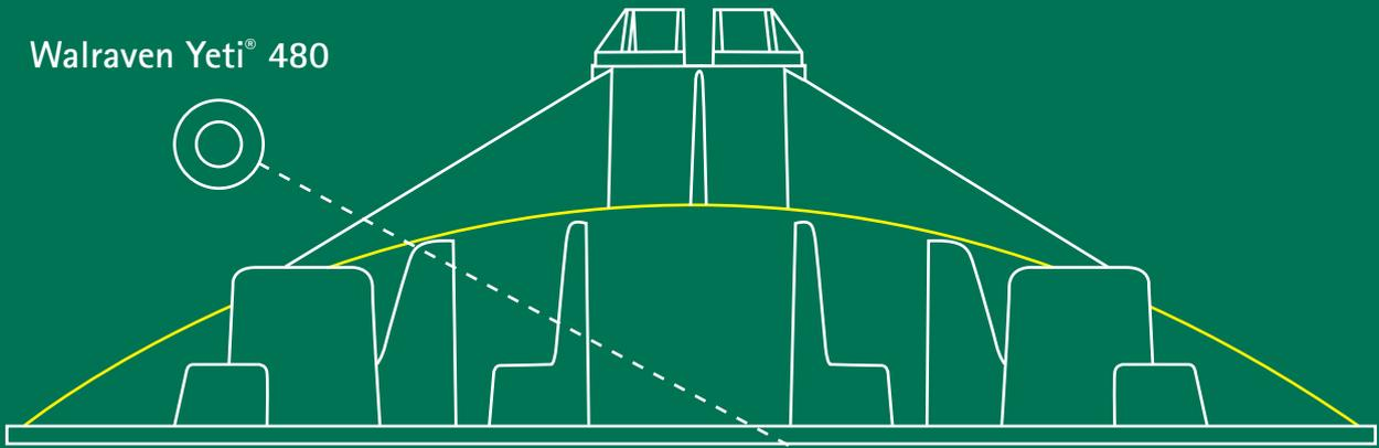
Adjustable to compensate roof pitch up to 7°
