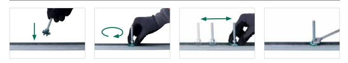
Our pre-assembled Walraven RapidRail<sup>®</sup> Hammerfix and Walraven RapidRail<sup>®</sup> Slide Nuts are 3 in 1 parts that simply push and twist into the rail.
