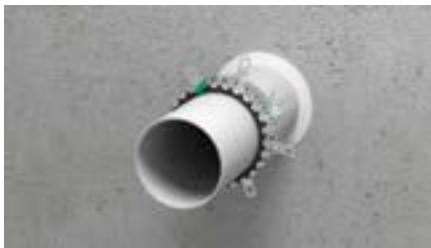
4. Close the collar by inserting the strip from the inside out through the second hole and bending it back.
