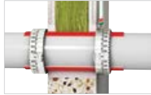
■ Built-in situation flexible walls \geq 100 mm
