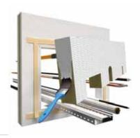
6. Seal the remaining aperture / joints with mineral fibre or fill them with Walraven Pacifyre® MWB-A.
