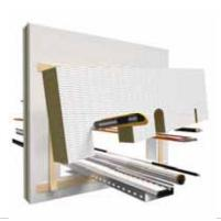
5. Coat the edges of the mineral fibre boards with Walraven Pacifyre® MWB-A and firmly place boards in position.
