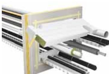
6. Seal the remaining opening/joints with mineral fibre or fill them with Walraven Pacifyre® MWB-A.
