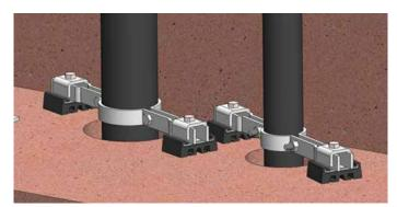
■ Whisper Riser Pads mounted to the floor or strut, mounting to strut raises the clamp for easy fire protection installation.
