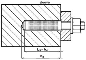
Installation of internal threaded socket with sieve
