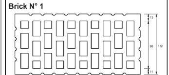
Hollow clay brick HLz 12-1,0-2DF according to EN 771-1 length/width/height = 235 mm/112 mm/115 mm  $f_b \geq$  12 N/mm² /  $\rho \geq$  1,0 kg/dm³
