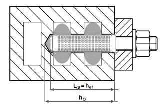
Installation of internal threaded socket with sieve
