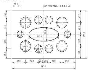
Hollow sand lime brick KSL 12-1,4-3DF according to EN 771-2 length/width/height = 240 mm/175 mm/113 mm  $f_b \ge 12 \text{ N/mm}^2 / \rho \ge 1,4 \text{ kg/dm}^3$
