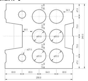
Hollow sand lime brick KSL 12-1,4-8DF according to EN 771-2 length/width/height = 250 mm/240 mm/237 mm  $f_b \geq$  12 N/mm² /  $\rho \geq$  1,4 kg/dm³
