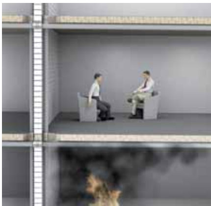
1. Fire breaks out in a fire compartment
