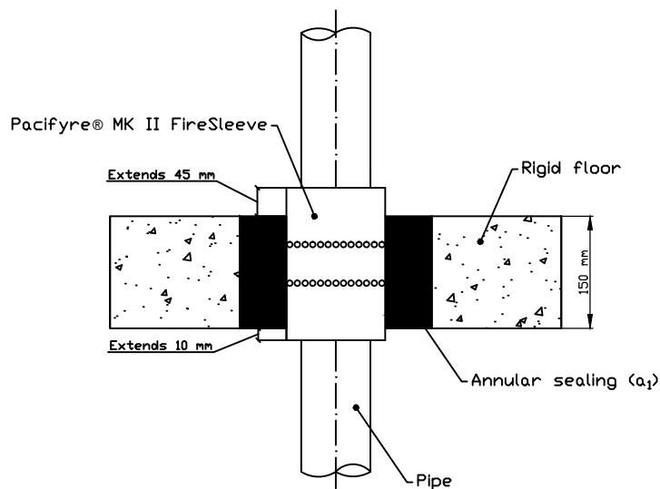
Drawing 2: single pipe penetration in a rigid wall construction.
