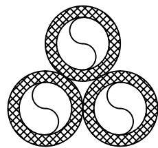
Drawing 6: single pipe penetration with zero distance in a rigid floor construction. Valid for seal variation i) with pipe separation  $a_2 = 0$  mm.
