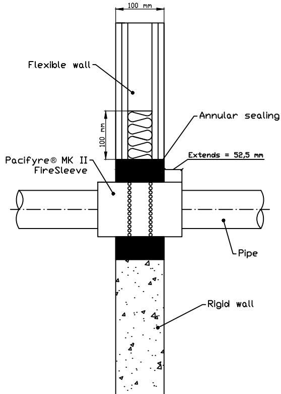
Drawing 4: single pipe penetration in a flexible or rigid wall construction.
