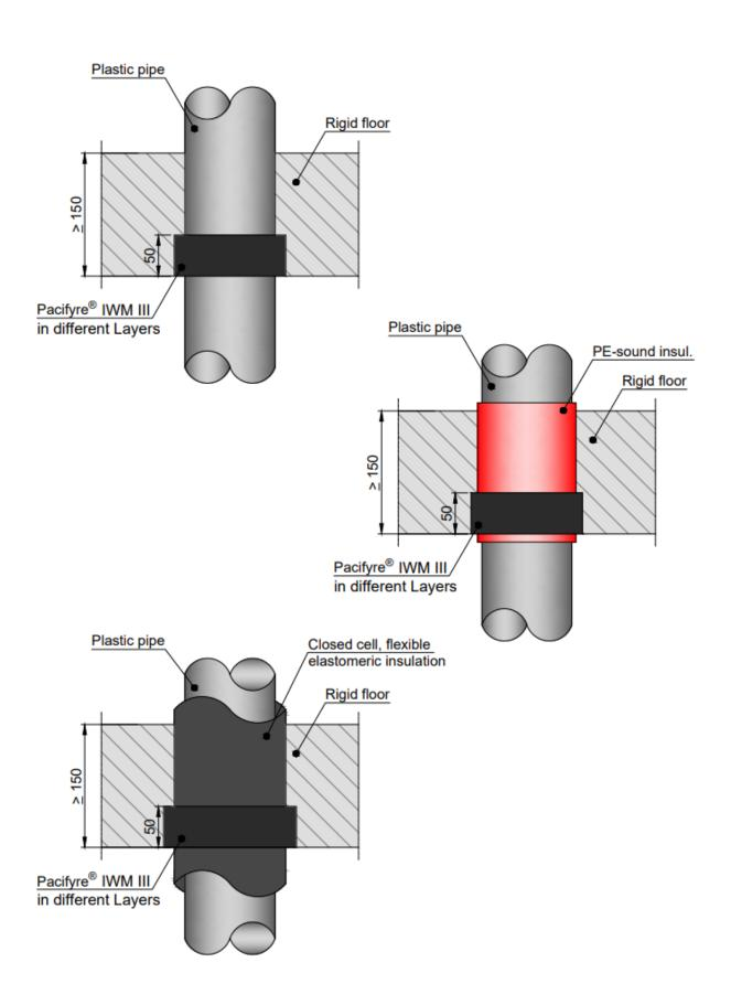
Installation in mineral wool sealants without additional pipe insulation
