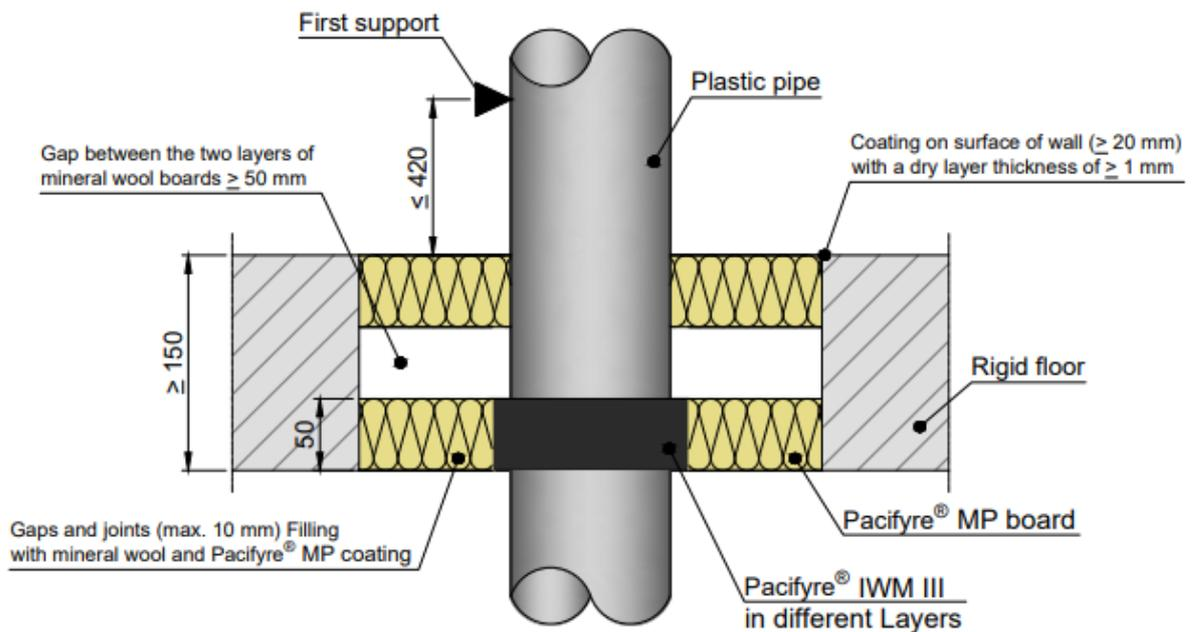
Installation in shaft wall partitions with or without additional pipe insulation
