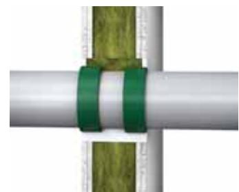
Penetration through flexible and rigid walls ≥ 100 mm.
