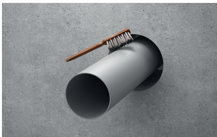
1. Clean the pipe and check the dimensions. Annular joint width max. 30 mm.
