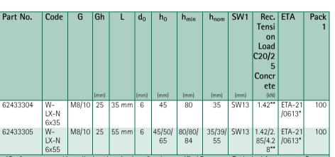
\*Performance and installation data is given for the specified European Technical Assessment. For full product data please refer to product data sheets. ETA-21/0612 according to EAD 330232-00-0601 anchoring in cracked and non-cracked concrete; ETA-21/0613 according to EAD
