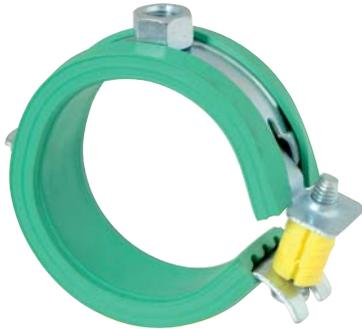
BISMAT® 5000 is a rubber lined pipe clamp uniquely designed for plastic pipe applications. This two-part clamp has a hinged side and the BISMAT® patented single screw quick locking system. The green EPDM rubber lining is UV resistant and is specifically designed to be smooth to allow for the expansion and contraction of plastic pipes.
