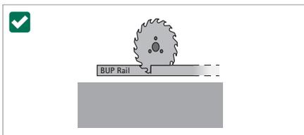
Because the BIS RapidStrut® (BUP1000) contains self repairing properties it is possible to cut the rail to length to meet your needs. The cut edges remain protected against corrosion. It may happen that some red rust is seen at the cut edges, which will disappear by the so called "self healing effect" within a time period of several months.
