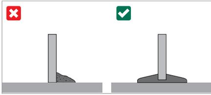
Design the system in such a way that there is no possibility of water or waste - organic or otherwise - stagnating around metal BIS UltraProtect® 1000 products. Use for example a BIS Yeti® or BIS Ursus to lift the BIS UltraProtect® 1000 System.
