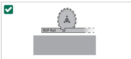
Because the BIS RapidStrut® (BUP1000) contains self repairing properties it is possible to cut the rail to length to meet your needs. The cut edges remain protected against corrosion. It may happen that some red rust is seen at the cutted edges, which will disappear by the so called "self healing effect" within a time period of several months.
