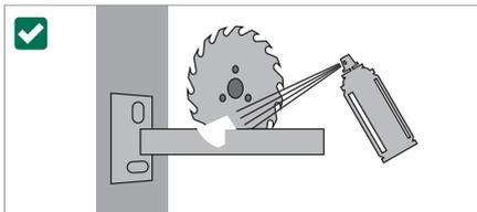
If you cut a cantilever arm or any other product from our BIS Ultra Protect® range, we strongly recommend that you treat the BIS UltraProtect® 1000 Cantilever Arms with the BIS UltraProtect®1000 spray set, as this will protect the cut edges in compliance with the BIS UltraProtect® 1000 requirements.
