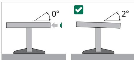
To make sure water runs off freely, place the BIS UltraProtect® 1000 parts at an angle of at least 2°. If leveled installations are required, make sure to fit the rail or cantilever arm with a BIS Rail End Cap (65660XX) for clean finishing of rail end and to cover all burrs. To prevent the accumulation of dirt inside the rail, use the BIS Strut PVC Profile (6566999) to close the slot (when fitted on top).
