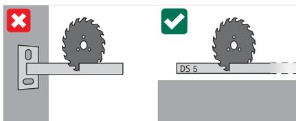
Because the BIS RapidStrut® DS 5 Fixing Rail contains self repairing properties it is possible to cut the rail to length to meet your needs. The cut edges remain protected against corrosion. We strongly advise that you do not cut the BIS UltraProtect® 1000 Cantilever Arms as this will leave the cut edges unprotected.
