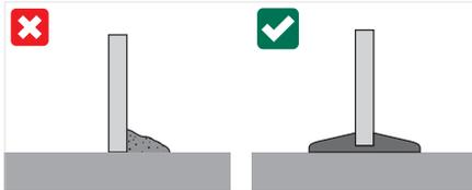
Design the system in such a way that there is no possibility of water or waste - organic or otherwise - stagnating around metal BIS UltraProtect® 1000 products. Use for example a BIS Yeti® or BIS Ursus to lift the BIS UltraProtect® 1000 System.
