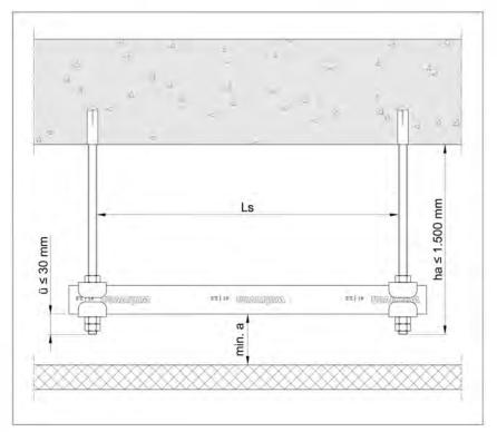
Minimum distance min.  $a \Rightarrow$  minimum distance between topside of a ceiling and underside of the mounting rail.
