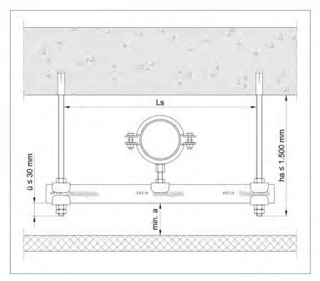
Figure 2: Example of a mounting rail combined with a pipe clamp installation in the ceiling plenum of a suspended ceiling construction in accordance with the Specimen Conduit Guideline [German designation: MLAR]), edition of 10/02/2015, Section 3.5.3
