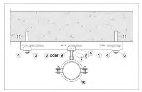
Figure: Execution as direct assembly
