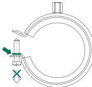
Anti-loss washers prevent screws from falling out
