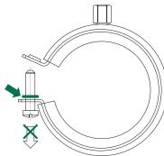
Anti-loss washers prevent screws from falling out
