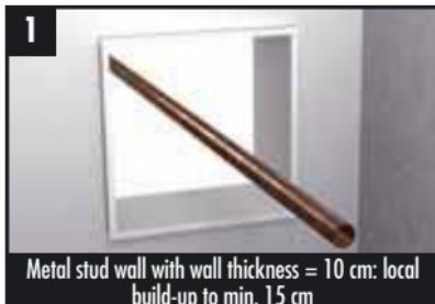
Metal stud wall with wall thickness = 10 cm: local build-up to min. 15 cm
