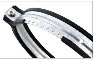
The rubber lining is formed around and through the steel band. It is conjoined with the steel and will not come off when sliding the spiral duct through the clamp.
